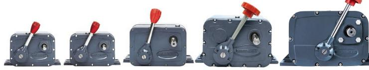
E Models 1, 2, 41 or 42 Torque Rating 12 in.lbs. Speed Range 0-400. Normal Input 1/4-1/3 H.P.
