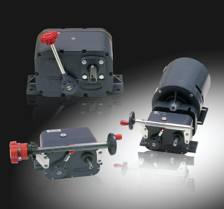
A Zero-Max Drive is a mechanical adjustable speed drive. Five sizes provide constant torque of 12 to 200 inch pounds throughout the speed range. The speed range is infinitely variable from 0 to 1/4 of the input speed under full rated load. This is generally stated as 0-400 RPM assuming an input of 1800 RPM.
